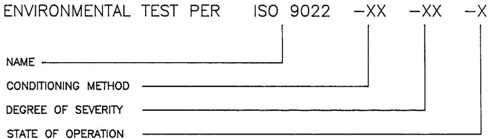
**FIGURE 1.27** Definition of an environmental test code which can be communicated in a one line call-out under ISO 9022.
