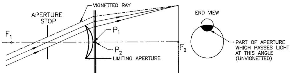
**FIGURE 1.7** Off-axis beam which is partially obstructed by a limiting aperture showing its vignetting effect and limiting the ultimate field of view.
