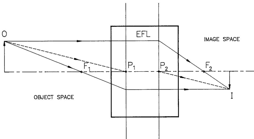
**FIGURE 1.4** Construction of an image point from a general object point to find the size and position of an image.
