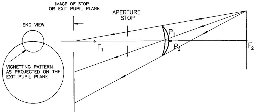
FIGURE 1.8 Construction of the vignetting pattern at a given field angle (image position) in image space.
