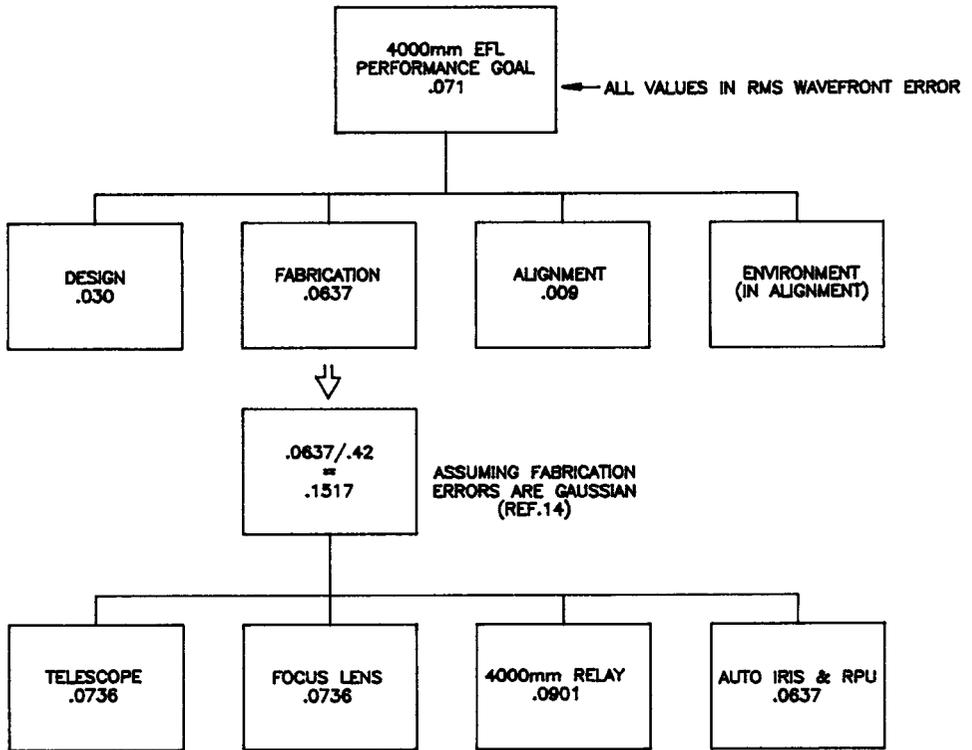
FIGURE 1.25 Error budget allocation for the 4000-mm channel of the multifocal length tracking telescope.
