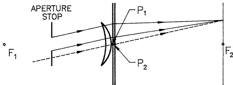
**FIGURE 1.6** Construction of the ray paths from an off-axis object through the aperture stop or pupil to the image plane.
