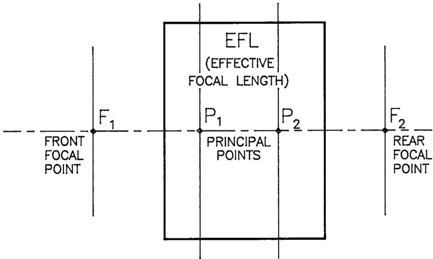
**FIGURE 1.3** The three properties which define a “Black Box” lens: effective focal length (EFL) and the two principal points (P<sub>1</sub> and P<sub>2</sub>).
