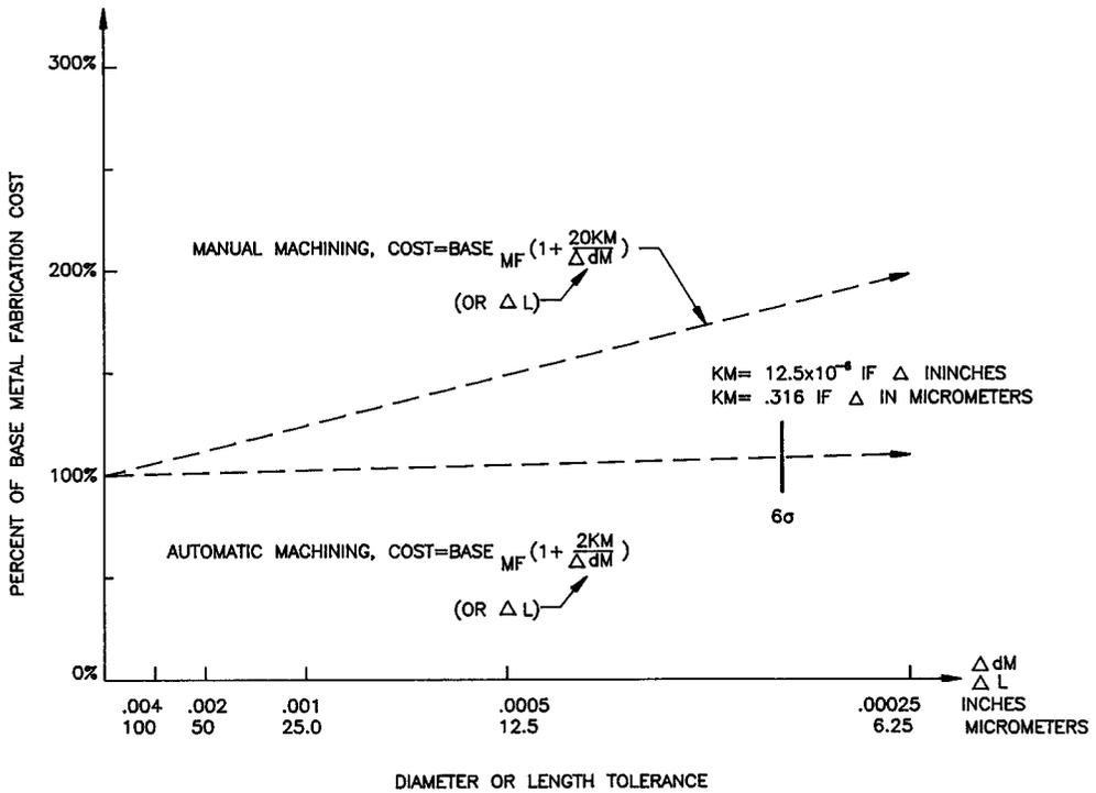
**FIGURE 1.19** Relative cost vs. reciprocal tolerance concerning lens bore diameters and lengths.
