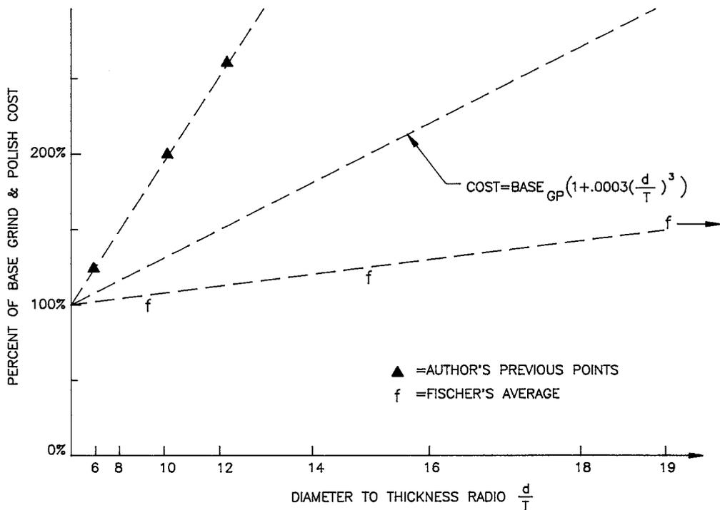
FIGURE 1.15 Relative cost vs. reciprocal tolerance according to various authors concerning lens diameter-to-thickness ratio.
