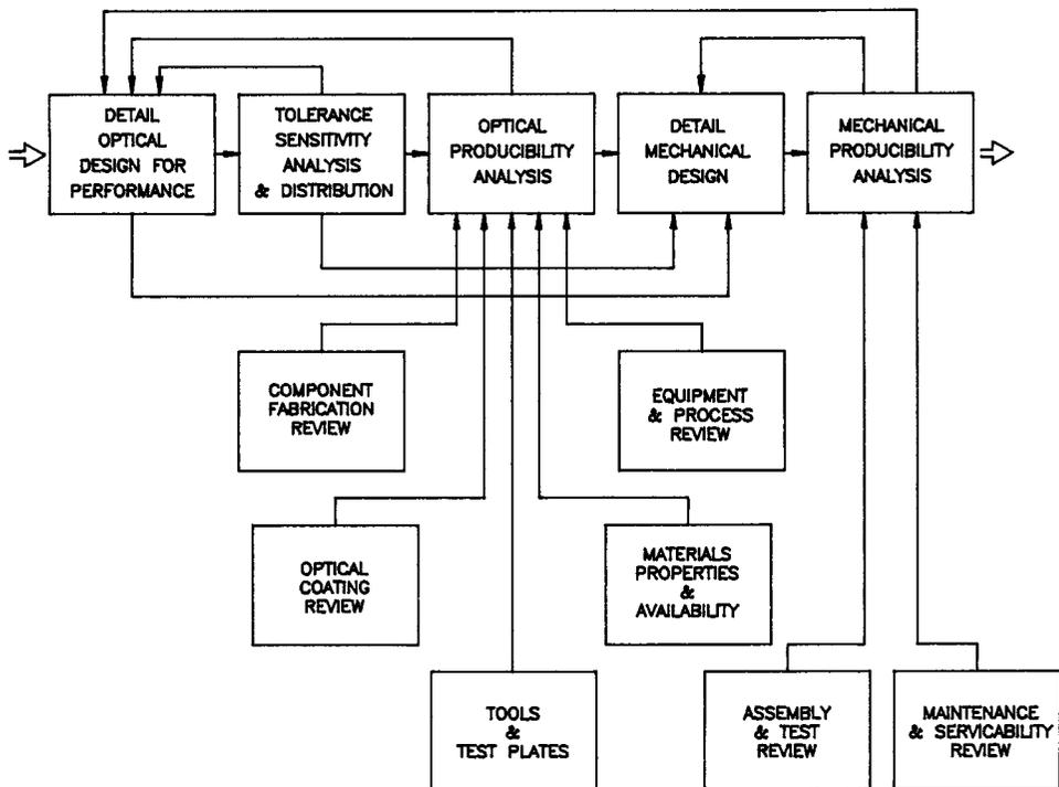
FIGURE 1.2 Detail design and analysis process of an optical product.
