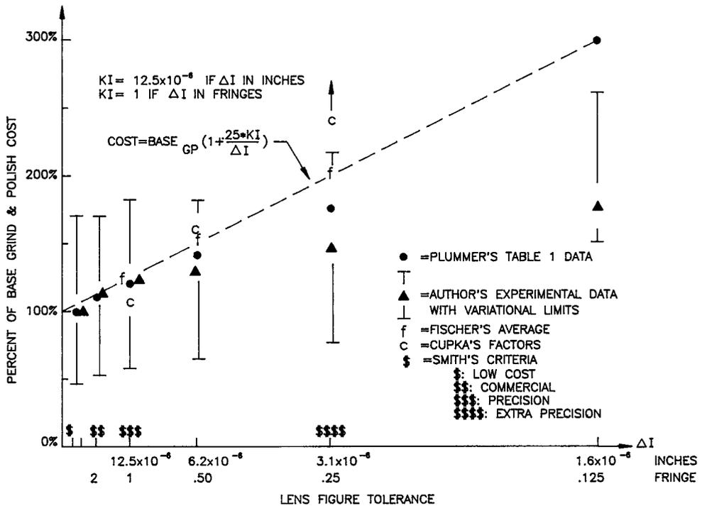
FIGURE 1.14 Relative cost vs. reciprocal tolerance according to various authors concerning lens figure irregularity.
