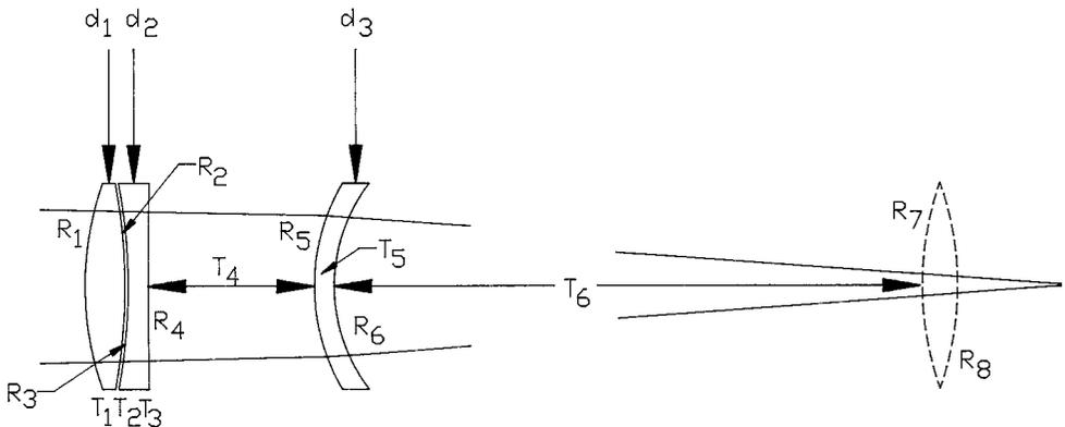
**FIGURE 1.26** Focus lens set of telescope used as an example.
