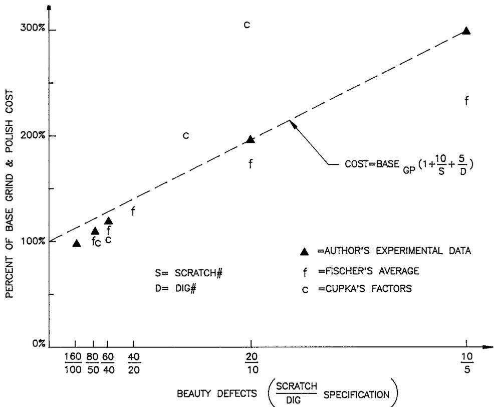
FIGURE 1.17 Relative cost vs. reciprocal tolerance according to various authors concerning surface finish or scratch and dig.
