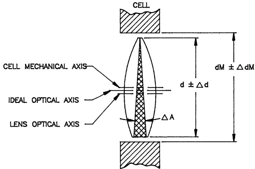
FIGURE 1.21 Decentering factors of a lens in a cell.
