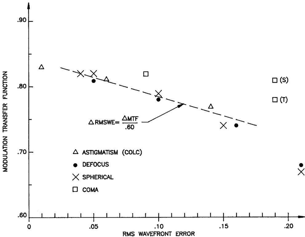
FIGURE 1.24 Diffraction MTF at 30 lp/mm vs. wavefront error for a 2000-mm, F/8 lens with various aberrations.
