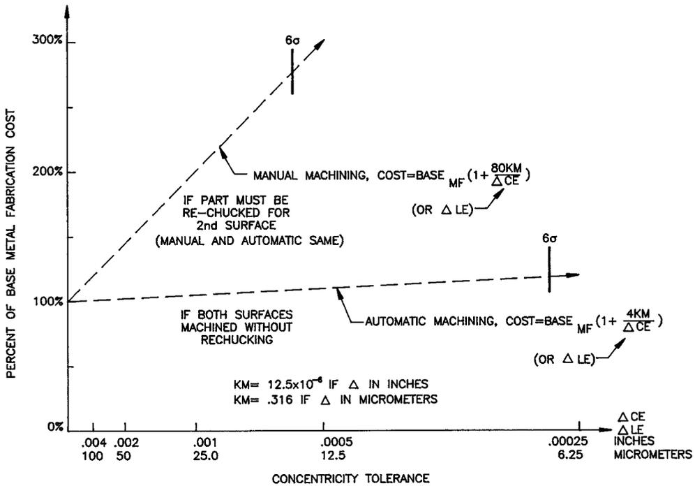
FIGURE 1.20 Relative cost vs. reciprocal tolerance concerning lens bore concentricity ( $\Delta CE$ ) and tilted and length run-out ( $\Delta LE$ ).
