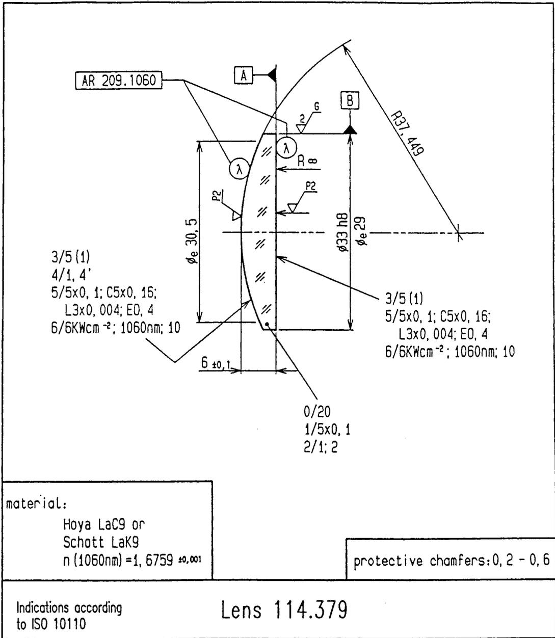
FIGURE 1.10 Example of a lens drawing to the ISO standards. Note the limited notes and dependence on any particular language (i.e., English).
