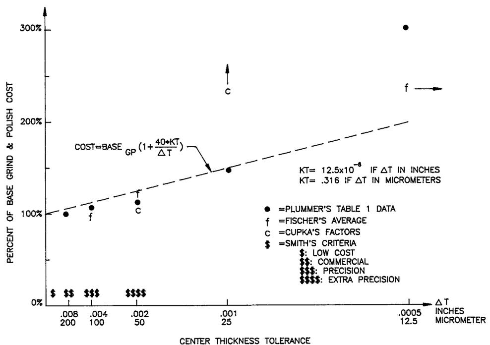
FIGURE 1.16 Relative cost vs. reciprocal tolerance according to various authors concerning lens center or axial thickness.
