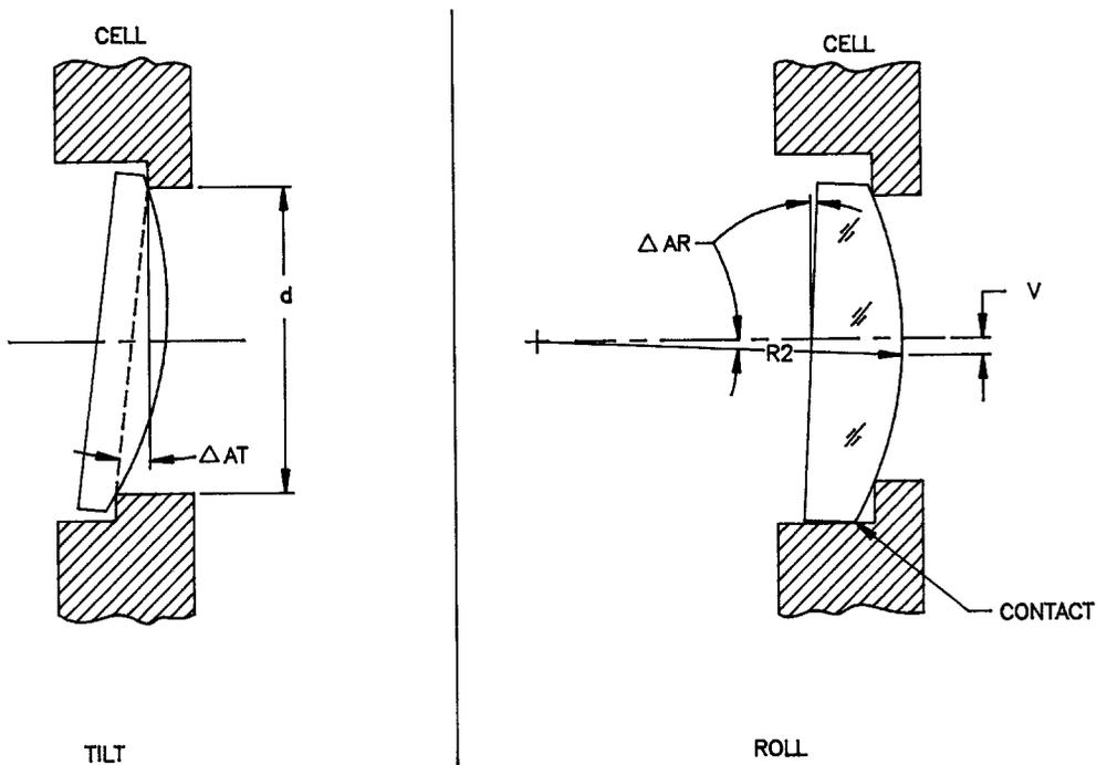
FIGURE 1.22 Tilt and roll factors of a lens in a cell.
