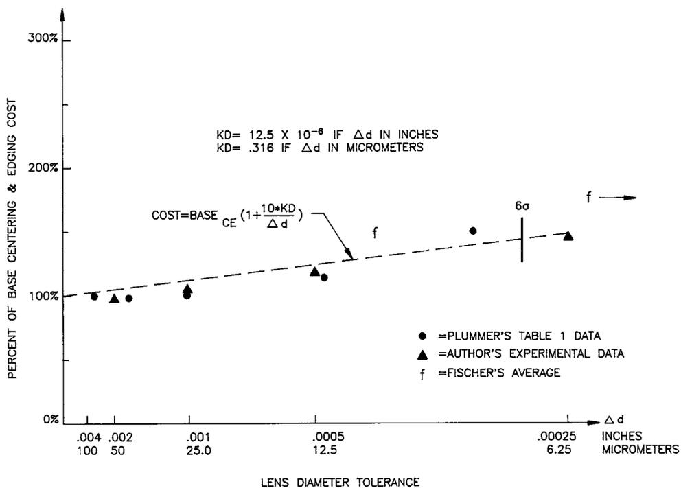
FIGURE 1.11 Relative cost vs. reciprocal tolerance according to various authors concerning lens diameter.
