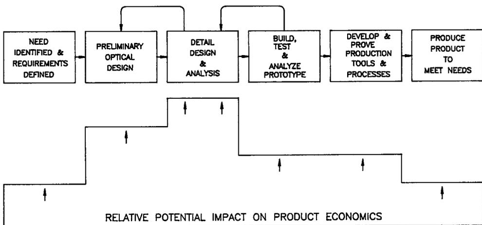
FIGURE 1.1 Overall process to develop and produce a new optical product.
