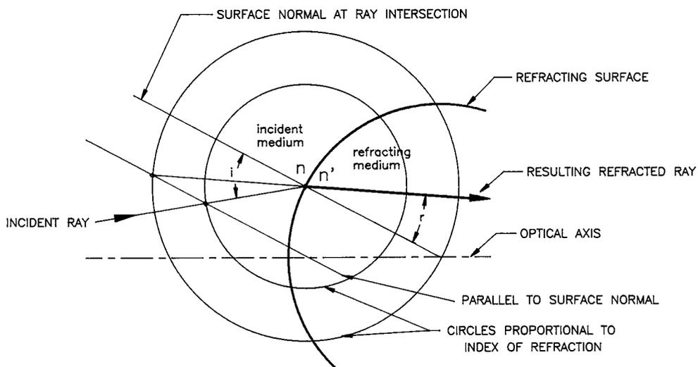
FIGURE 1.9 Rigorous ray tracing by construction of a refracted ray.
