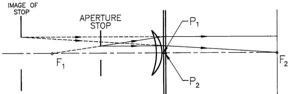
**FIGURE 1.5** Finding the exit pupil of a system by constructing the image of the aperture stop.
