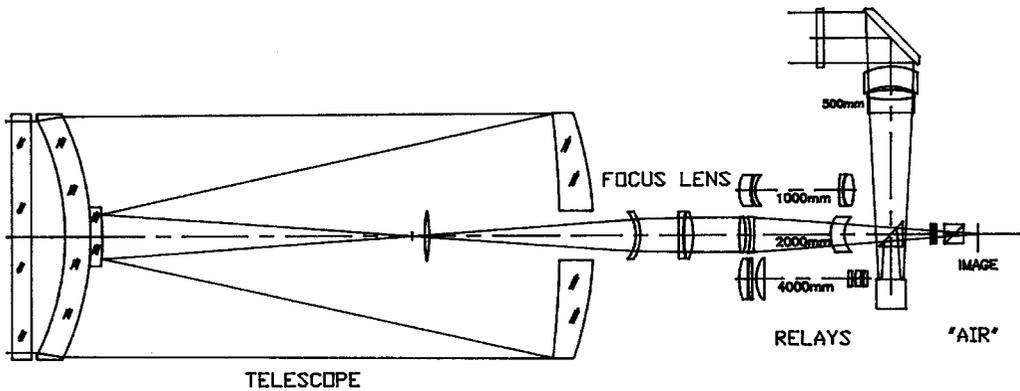
FIGURE 1.23 Example system: Multifocal length tracking telescope.
