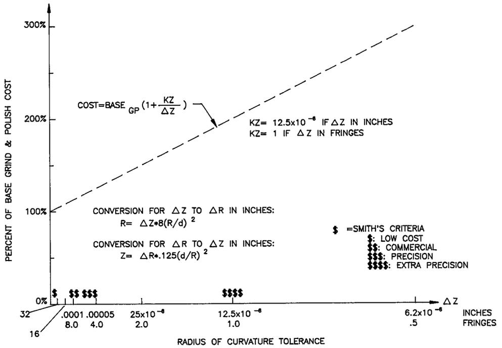
FIGURE 1.13 Relative cost vs. reciprocal tolerance according to various authors concerning radius of curvature (when expressed as sagittal error).
