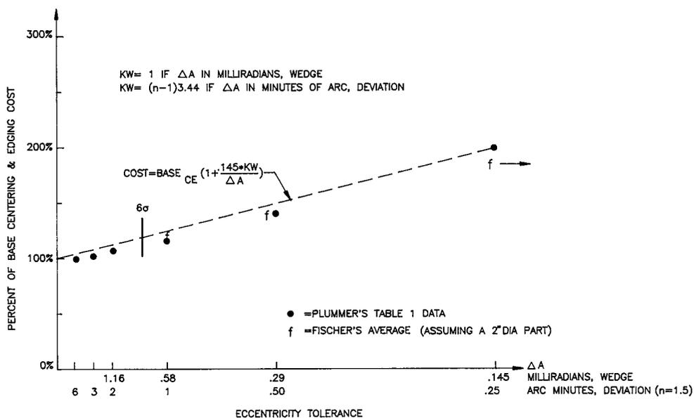
FIGURE 1.12 Relative cost vs. reciprocal tolerance according to various authors concerning eccentricity.
