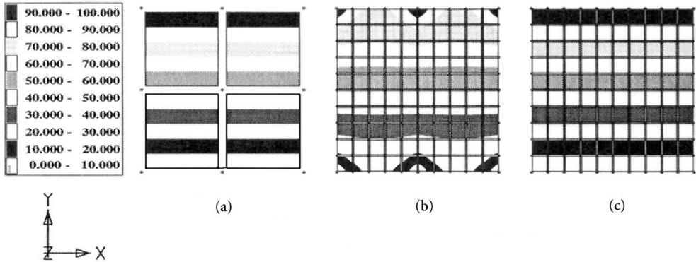
**FIGURE 9.8** Interpolation of temperatures from coarse to detailed model. (a) Temperatures determined from coarse model; (b) interpolated temperatures by conduction model; and (c) interpolated temperatures by shape functions.
