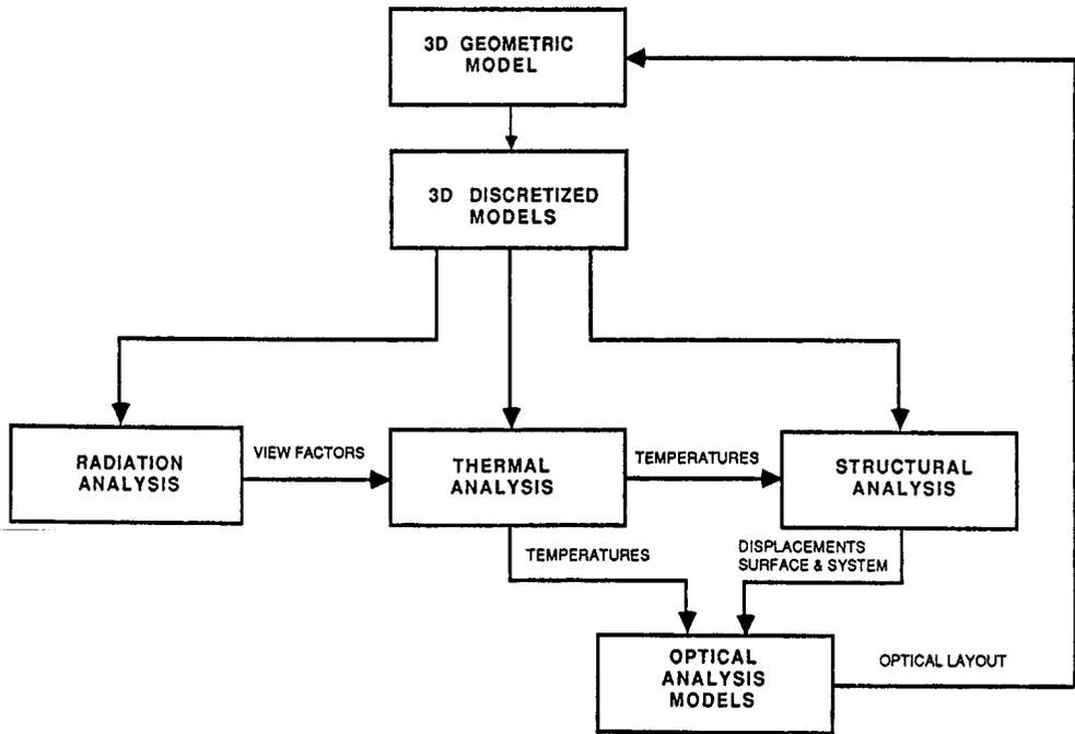
FIGURE 9.1 Data flow in optomechanical design.
