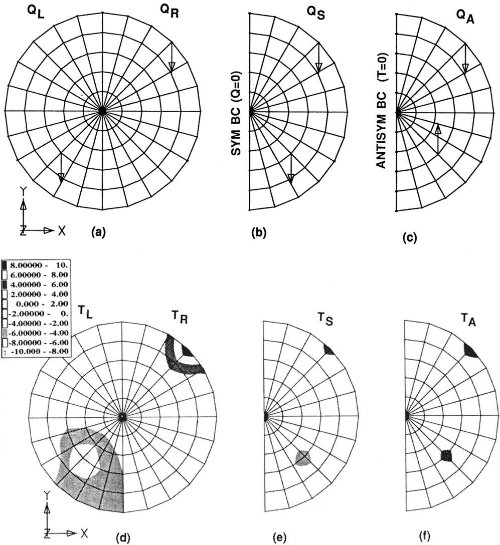
**FIGURE 9.5** Thermal analysis of a symmetric structure with asymmetric loads. (a) Full model with general loads ( $Q_R$  and  $Q_L$ ); (b) half-model with symmetric loads ( $Q_S$ ) and boundary conditions; (c) half-model with antisymmetric loads ( $Q_A$ ) and boundary conditions; (d) full model with temperature results ( $T_R$  and  $T_L$ ); (e) half-model with symmetric temperatures ( $T_S$ ); (f) half-model with antisymmetric temperature ( $T_A$ ).
