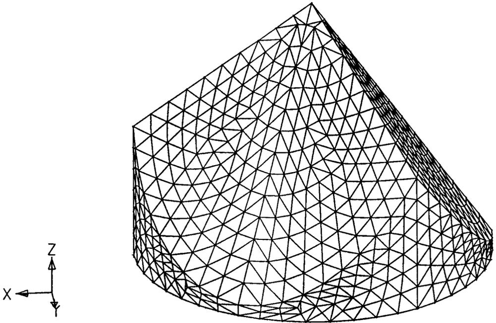
FIGURE 9.7 3D model of a corner cube.
