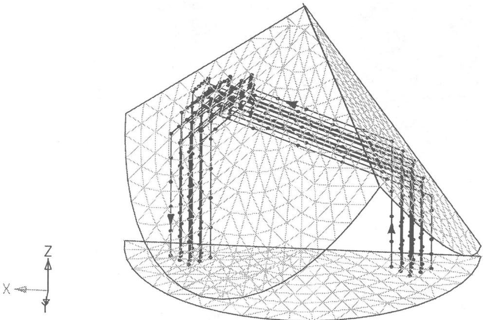
**FIGURE 9.14** Individual beam paths in a corner cube represented as rod elements.
