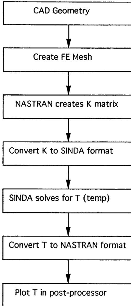
FIGURE 9.4 Thermal analysis flowchart.
