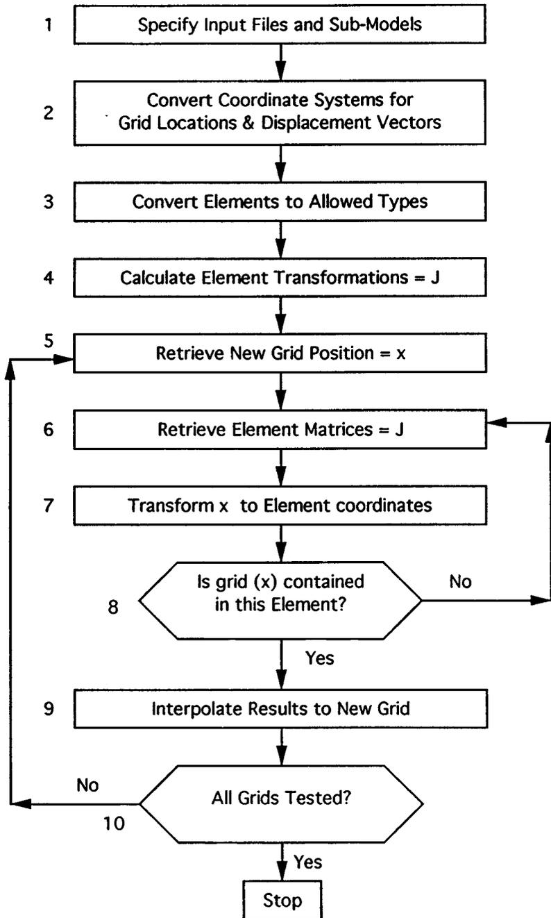
FIGURE 9.9 Flow chart for shape function interpolation.
