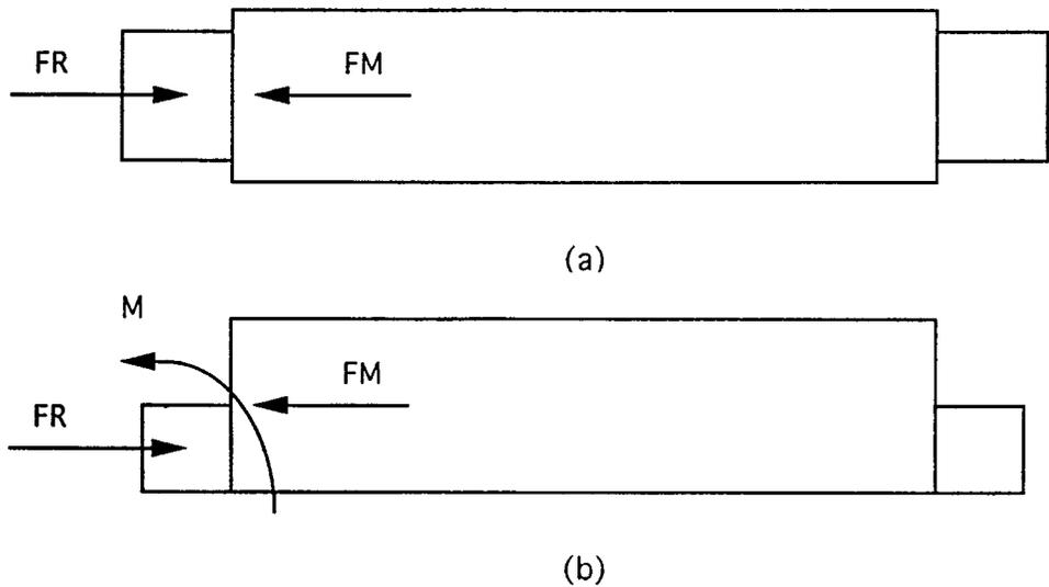
**FIGURE 9.11** Line of action comparison on a mirror and mount ring. (a) Ring aligned with neutral axis and (b) ring unaligned with neutral axis.
