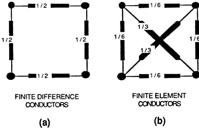
FIGURE 9.3 Conduction links for a square mesh. (a) Finite difference conductors; (b) finite element conductors.
