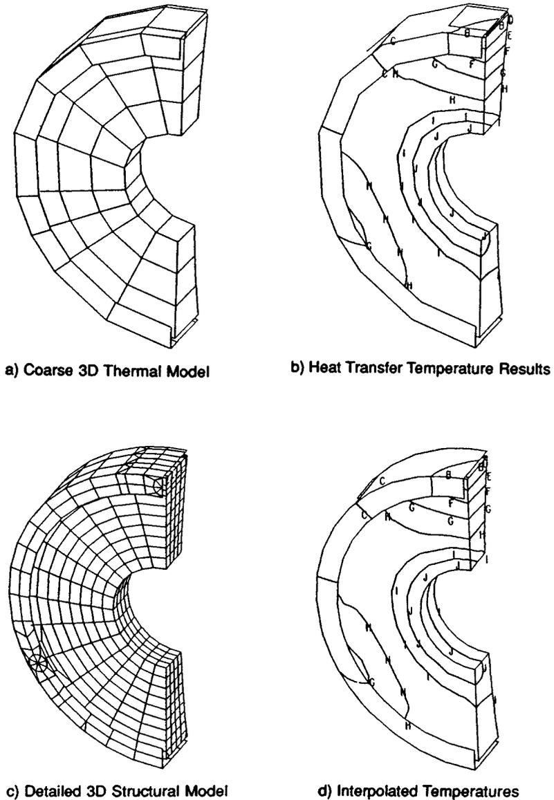
**FIGURE 9.10** Shape function interpolation on a mirror and mount ring. (a) Coarse 3D thermal model; (b) heat transfer temperature results; (c) detailed 3D structural model; and (d) interpolated temperatures.
