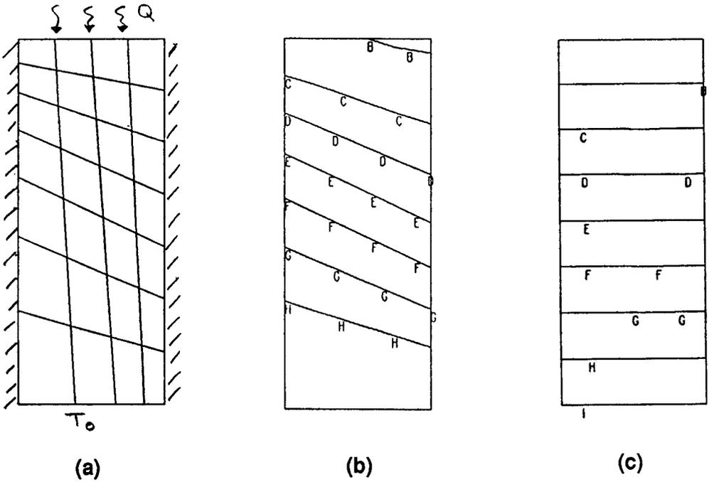
FIGURE 9.2 Simple heat conduction example. (a) Skewed mesh pattern; (b) finite difference results; and (c) finite element results.
