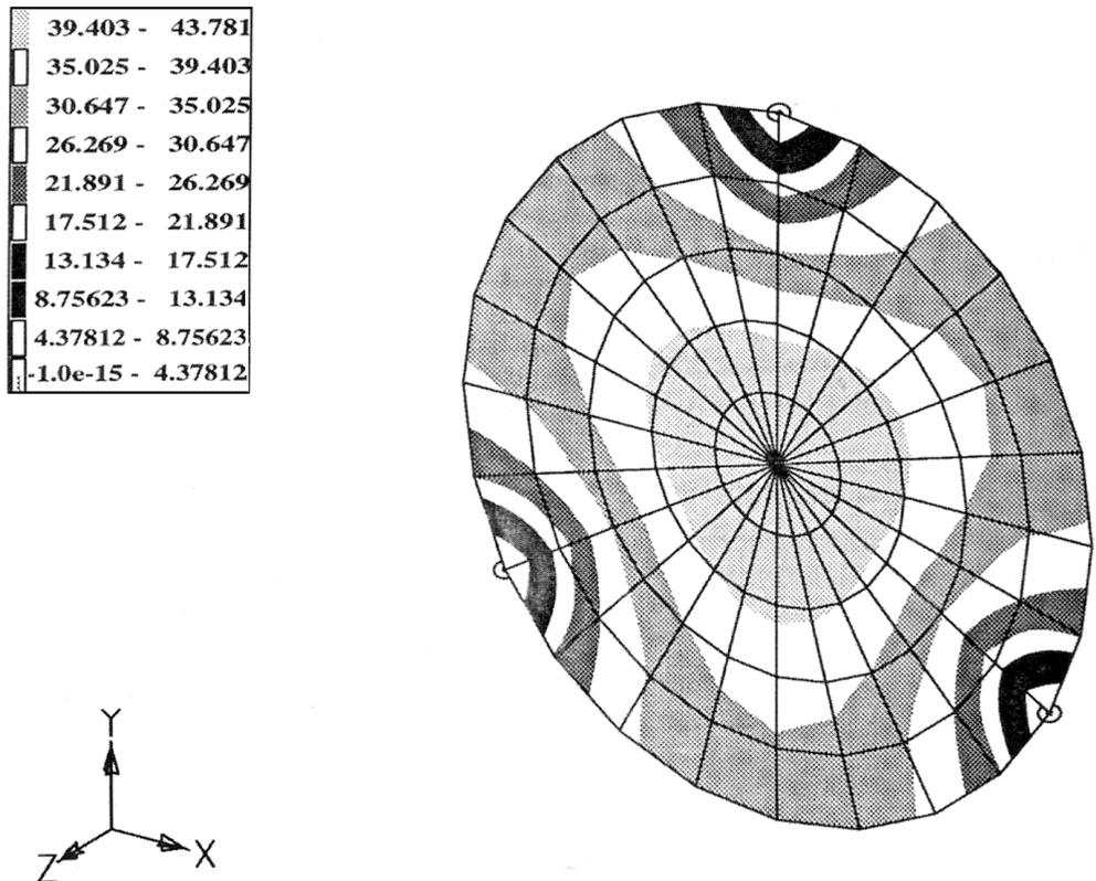
FIGURE 9.6 2D model with in-plane temperature contours.
